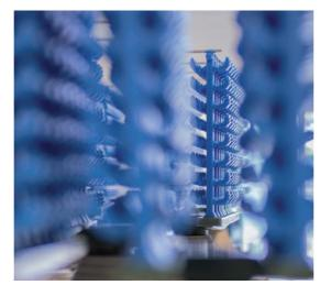
Our lost-wax casting process can be used to do away with the need for finishing operations and produce **complex** geometries with high dimensional accuracy and superb surface
