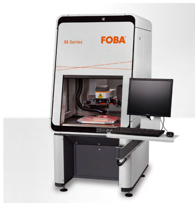
Laser marking machine with integrated vision system for inspection steps before and after marking.
