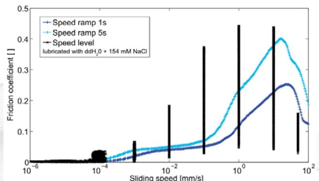
Figure 7: The measuring accuracy depends on the rotational speed. Friction measurement results obtained from speed ramps and from measurements at constant speeds are compared.
