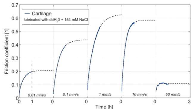
Figure 6: Cartilage friction over time at different rotational speed levels.
