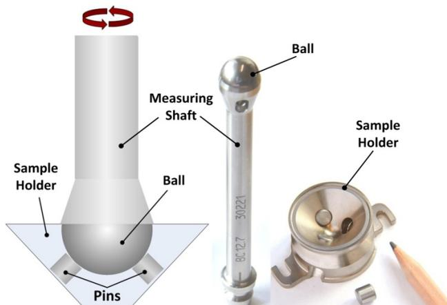
Figure 2: Schematic illustration of the tribological test setup probing a set of three osteochondral cylinders with a ½-inch glass sphere.
