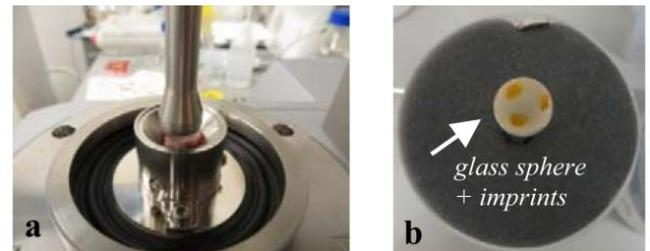
Figure 4: Tribology setup with mounted sample holder and lowered measuring head (a) and evaluation of the contact area between cartilage surface and glass sphere (b).
