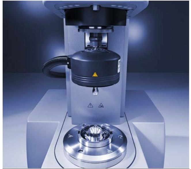
Figure 3: Anton Paar MCR with a tribological measuring cell.
