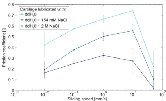
Figure 8: Comparison of cartilage friction using lubricants with differences in their ionic strength.
