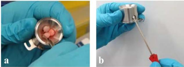
Figure 1: Sample holder setup: 3 cylindrical samples are placed into the sample holder (a) and their vertical position is adjusted with set screws (b).
