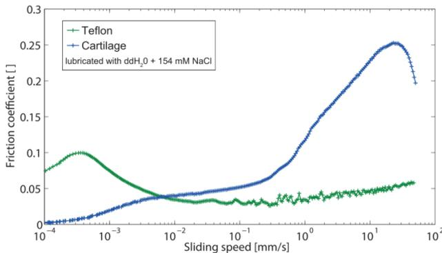
Figure 5: Comparison of friction coefficients measured for PTFE plates and cartilage samples against a glass sphere.
