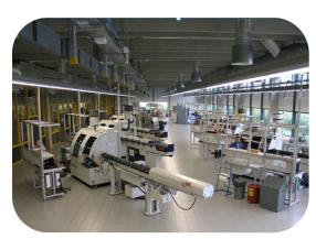
The **turning & milling** workshop has a series of CNC and EDM machines. Each work bench is equipped with measuring instruments for controlling, at any time, the quality of the products manufactured.
