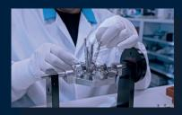
The size of parts and the required precision necessitate a controlled atmosphere in the entire assembly workshop, with continual air change and filtration. A clean room ISO 7 is
