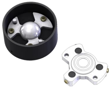
Figure 3 - Clamping parts of the sample holder: lower support (left) and upper clamp (right). Note three magnetic pegs for firm holding between the two parts.
