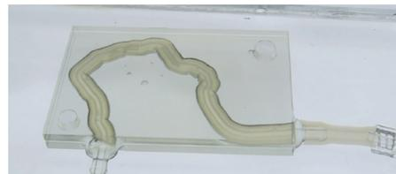
CSI 3D prints coronary blend plates using PolyJet technology.
