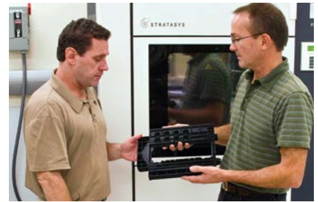
This prototype was created with the FDM process. It helped optimize the design for injection molding.
