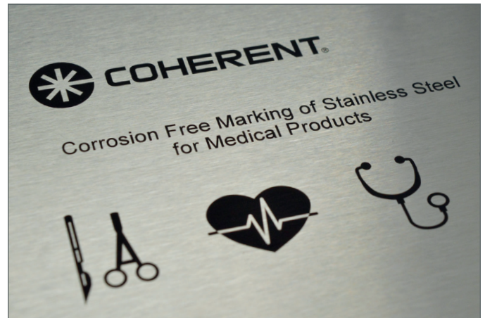
Figure 2. Black marking creates high contrast permanent marks in stainless steels such as this 1.4301 example.
